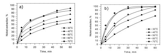
Fig. 2. Effect of temperature on nickel extraction in 2.0 M HCl: a) RANG-19 b) KUB-3.
